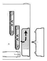
3. Replace the battery compartment door.
